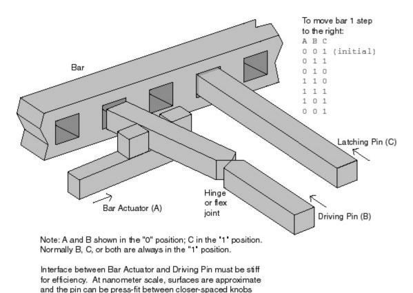
Fig. 2. A schematic of a thermodynamically efficient repositioning system.
