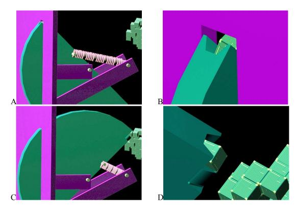
**Fig. 5**. A) The manipulator is in position to gather a block from solution. B) A close-up of the socket's position with a block inserted. C) The manipulator has moved to attach the block to the product. D) A close-up of the block about to be pressed into place.
