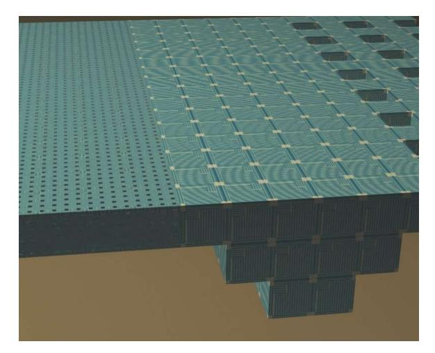
**Fig. 7**. A water filter with .3 nanometer pores (on left) would clean water down to the atomic level with minimal pressure drop due to drag. Such thin membranes would need to be supported by struts (center). Larger pore sizes are possible (on right). The very smooth surface on top would reduce fouling.
