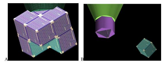
**Fig. 4**. Two ways to implement a socket: A) Place several blocks to form a cavity, perhaps followed by post-processing to modify the inner faces. B) Use a special-purpose molecular building block.
